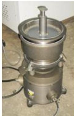
Figura 4.14 – Reômetro BTRHEOM
