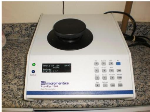
Figura 3.3 – Picnômetro a gás Accu Pyc 1340 (Micromeritics)
