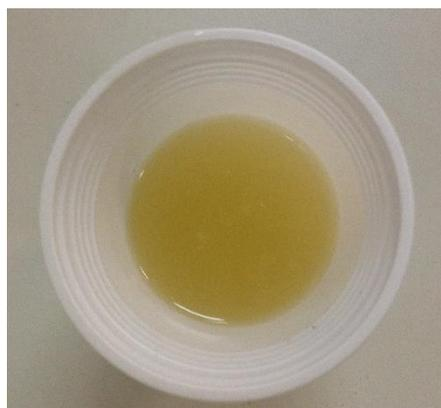
Figura 3.25 – Superplastificante Glenium 51
