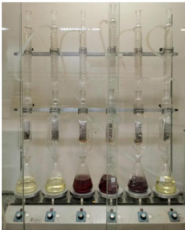
Figura 3.9: Extrator de Soxhlet
