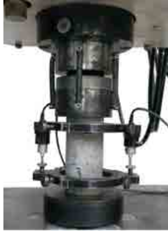
Figure 4.7: Compression test with LVDT attached.
