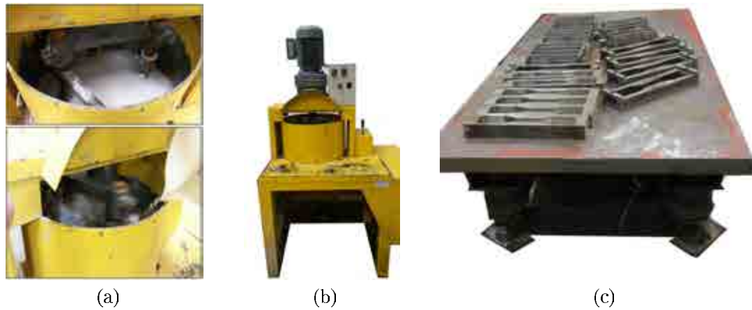
Figure 4.3: a) Concrete being mixed; b) Vertical planetary mixer; c) Moulds on the vibration table, before pouring the concrete.
