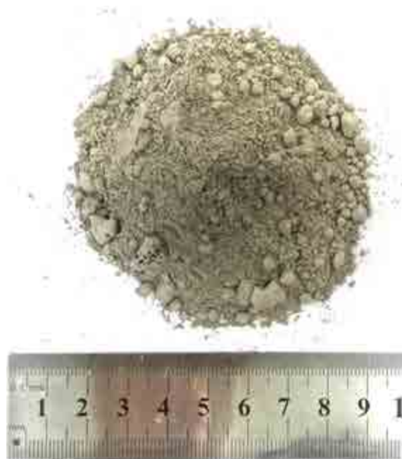
Figure 3.1: Dense refractory concrete, Brasilcast 560, without water addition.
