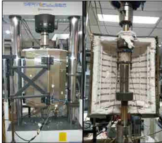
Figure 4.8: Press SHIMADZU EH-FM300K1-070-0A , showing the kiln and the test set up apparatus.
