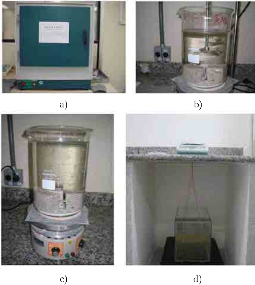
Figure 3.8: a)Kiln for drying samples, determination of the dry mass ( m_d ); b) Water heating; c) Sample saturation; d) Hydrostatic balance and determination of the immerse mass ( m_i ).
