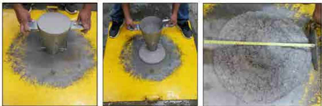
Figure 4.4: Inverted slump test procedure.
