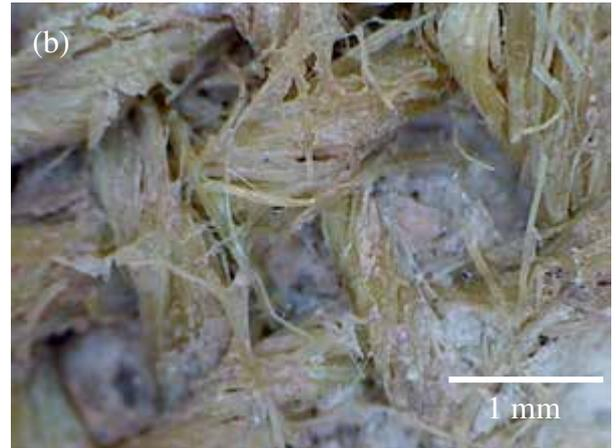
Figure 9. Images from a stereo-light microscope for MK matrix samples: (a) Uncoated fiber and (b) Coated fiber – Reference matrix.
