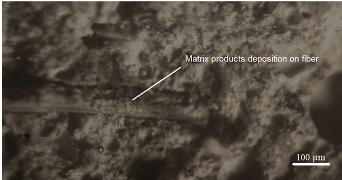
Figure 6-17 Matrix products deposited on curauá fiber.
