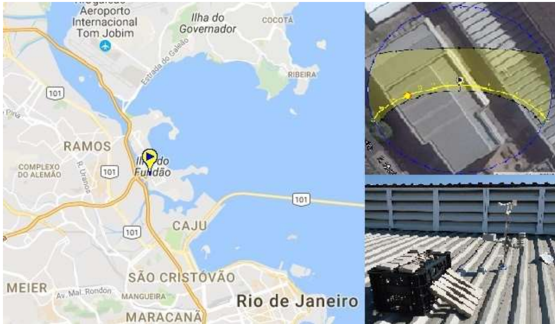
Figure 6-1 Location of natural weathering tests with sun path and specimens exposition on the roof (SunEarthTools.com).
