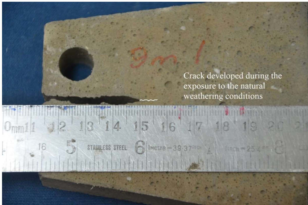
Figure 6-8 Crack developed during the exposure to natural weathering conditions.
