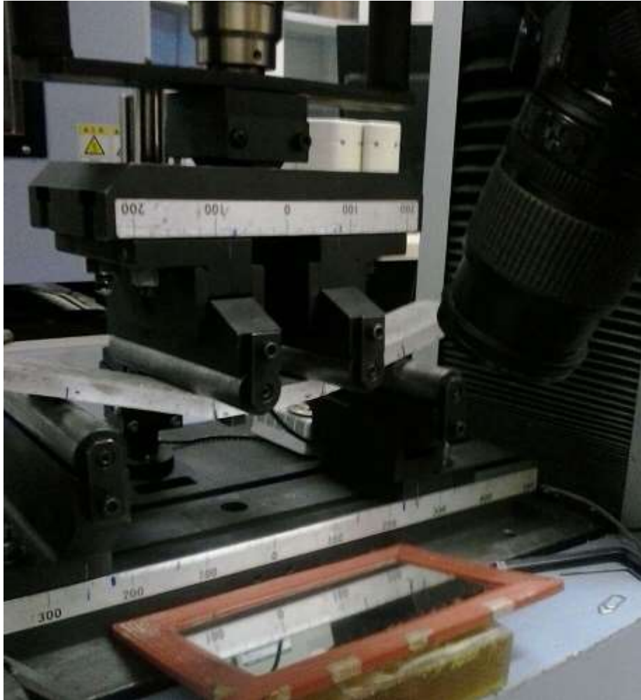
Figure 5-9 The 4-point bending test with the middle span deformation span controlled by LVDT, camera image used for crack pattern analysis.
