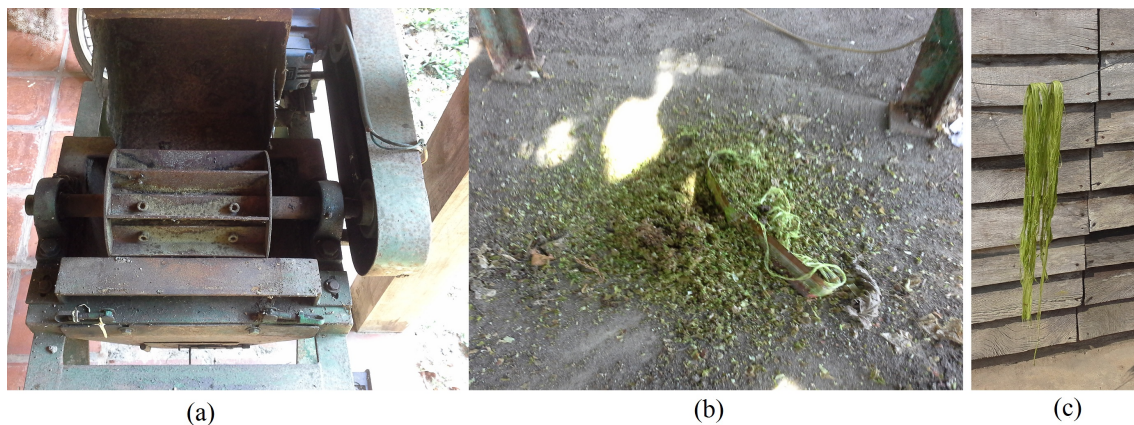
Figure 2-18 Curauá fiber extraction, (a) machine used to fiber separation from leaves, (b) mucilage (residue after fiber extraction), (c) curauá fiber drying in the sun.
